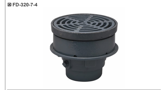
FD-320-7-4 Epoxy coated, cast iron body, body collar with weepholes and membrane clamp, trap primer connection with plug, anchor flange, no hub outlet.
