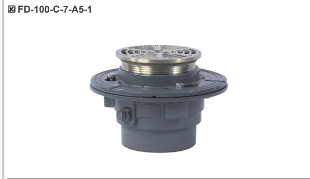
FD-100-C-7-A5-1 Epoxy coated, cast iron body, reversible flashing clamp with primary and secondary weepholes, trap primer connection with plug, no hub outlet.
