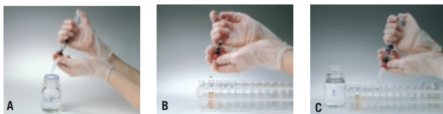
Fig 5. Using a GSTrap FF column with a syringe. A) Prepare buffers and sample. Remove the column's top cap and twist off the end. B) Load the sample and begin collecting fractions. C) Wash and elute and continue collecting fractions.
