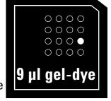
chip well when dispensing. This prevents a large air bubble forming under the gel-dye mix. Placing the pipette at the edge of the well may lead to poor results.
